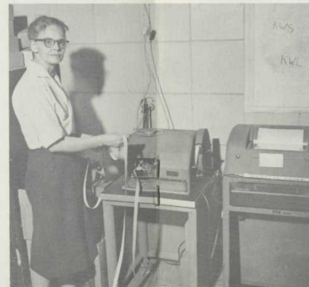
BILLING DATA is supplied from warehouses throughout the U.S. on facsimile punched tape sent over Sylvania private teletype machine, and checked here by Marguerite Fisher.
