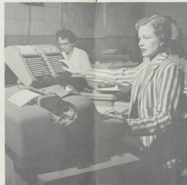
Mary Jane Alexander concentrates on accuracy as she operates Cardatype Machine for rapid processing of dealer order. Same type equipment is used in Ann Arbor and six field warehouses. Machine automatically types repetitive information, while Mary Jane adds variable quantities.
