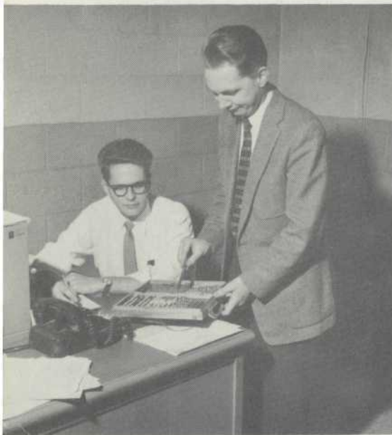
CARDATYPE CONTROL is established by maze of electronic connections in control panel shown here being adjusted by Herb Wick-ersham and Joe Rasmussen. Machine can be used for a variety of punch card assignments by changing control panel set-up.
