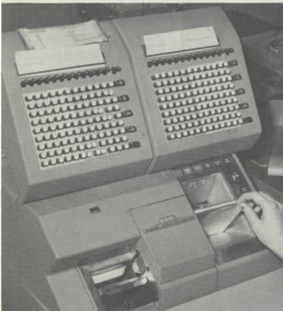
PRODUCT CARD is inserted in Cardatype Machine to control automatic typing of model number and product description on "shipper" documents which tell warehouse how to pack order. Push buttons on machine are used by operator to provide details of quantities ordered, shipped and back-ordered.
