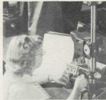
Histogram Methods and Irene Root uses histogram equipment are used in inspecting glass blanks by Grace Drechsel.
